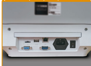
Full interface (Micro SD, USB, LAN, Dual RS232)
